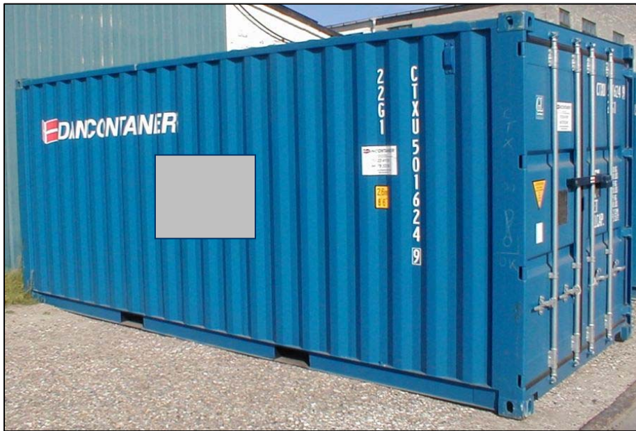
Figure 4: A 20-foot container showing the location of the plastic eWall™ panel.
